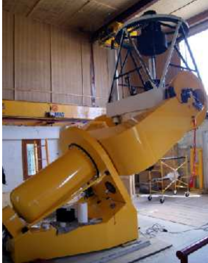
Figure 5. A view of 1.3m optical telescope, installed at Devasthal.
