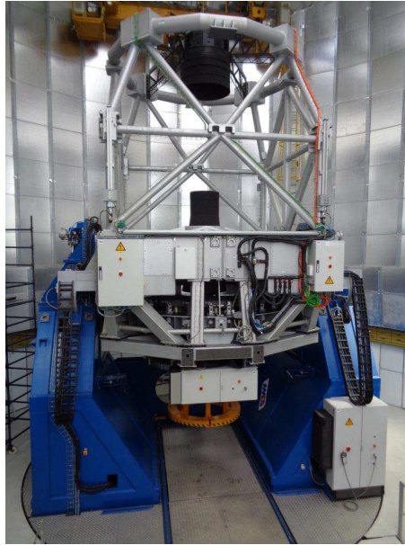
Figure 2. A picture of 3.6m Alt-az telescope from inside the dome. The height of telescope is about 11m. The forks are seen in blue color.
